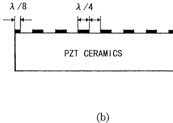
Fig. 11. (a) Electrode arrangements of a 40-MHz BGS wave resonator and (b) cross-sectional view of the resonator.
